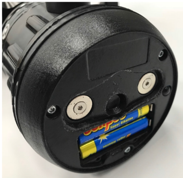
Figur 43: Dysebatterier bag tracking-pucken
