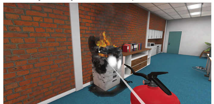
4. Discharge the extinguisher within its effective range using the P.A.S.S. technique (pull, aim, squeeze, sweep). Back away from an extinguished fire in case it flames up again
